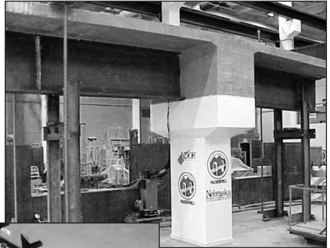
Above - New splice details for steel girder bridges were shown to guests at the University of Nebraska Engineering Lab.
