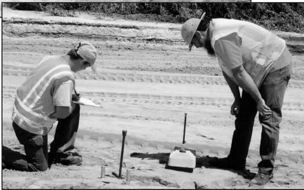
Above - After completing compaction of the subgrade with heavy machinery, maintenance personnel (below) check the compaction with a nuclear density gauge.
