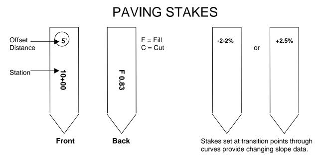
Fill (cut) is to the top of the pavement at outside edge.
