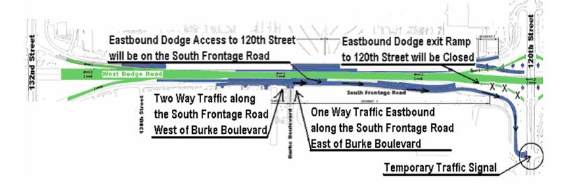
This Ramp relocation is necessary to construct piers for the Eastbound Elevated Expressway Bridge.
