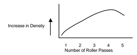
This example shows that the maximum density is achieved after 4 roller passes. You may want to record the nuclear readings after each pass of the roller and do some follow up readings to see if any changes in the rolling pattern are needed.
