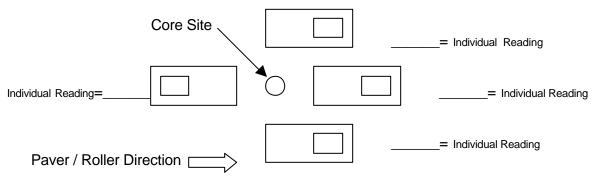
Note: Not to scale, nuclear gauge will be placed directly adjacent to core hole.
