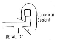
For the concrete girder design, concrete sealant shall also be applied to the outside face and bottom flange of the exterior girders as shown in Detail 'B'. Color shall match number 30045 of Federal Standard No. 595B.
