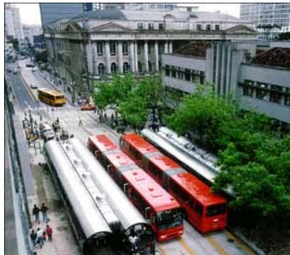
Capacity can be increased by using articulated, and even (in Curitiba) double-articulated buses. However, a limitation of buses compared to all other options, is that they cannot be coupled into trains. Buses must be run more frequently than fixed guideway systems to achieve high PHPD capacity.
